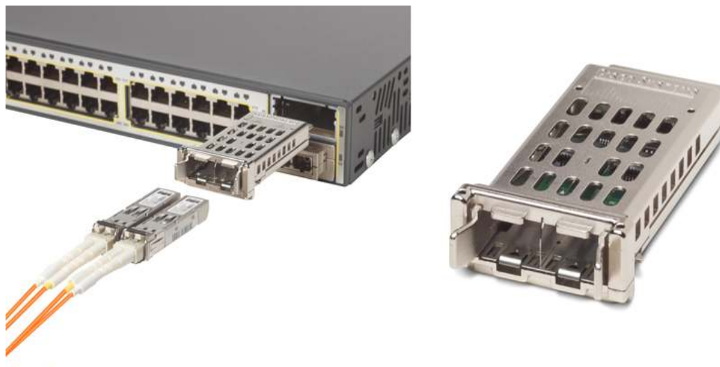
Figure 3. Cisco TwinGig Adapter Converting 10 Gigabit Ethernet X2 Interface into Two Gigabit Ethernet SFP Interfaces
