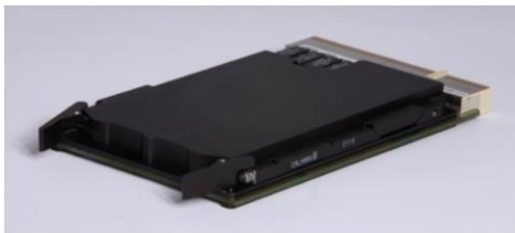
Figure 2. Cisco 5940 ESR—Conduction-Cooled Model
