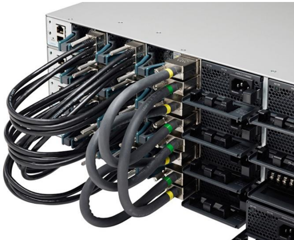
Figure 5. StackWise-480 and StackPower Connectors
