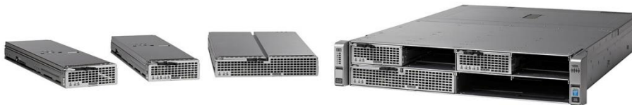
Cisco UCS M4308 Modular Chassis Supports Cisco UCS M142, M1414, and M2814 Compute Cartridges
