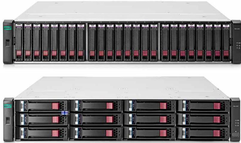
HPE MSA 2042 Storage offers an entry storage platform with built-in hybrid flash for application acceleration and high performance. It is ideal for performance-hungry applications and includes 800 GB of solid-state drive (SSD) capacity.
